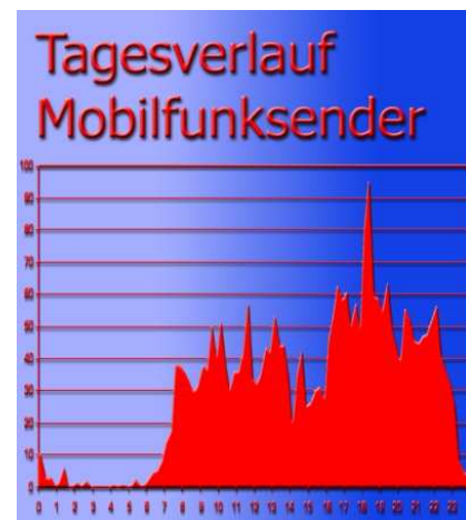
Daily variation of this RF transmitter discloses EXTREME variation in time
